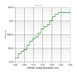
Delay time ranges from 0V to 25% VDD. The delay time comes to maximum when it exceeds 25% VDD
