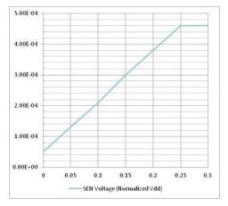
Take out R2, C5. The detecting distance reaches the longest when R7 is  $0\Omega$ . Sensitivity ranges from 0V to 25% VDD.
