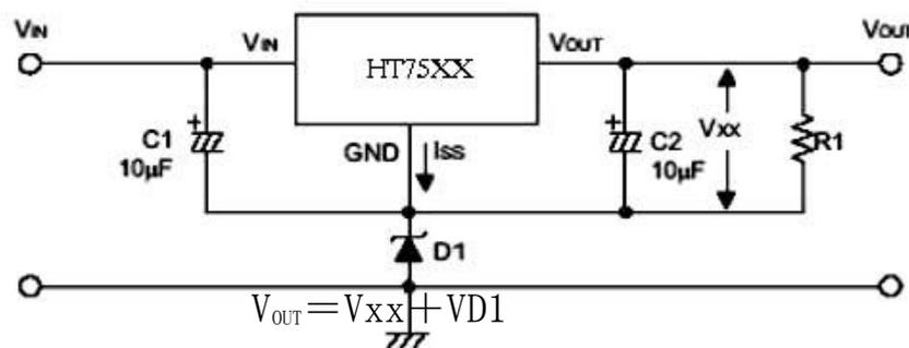
$$V_{OUT} = V_{XX} + V_{D1}$$
