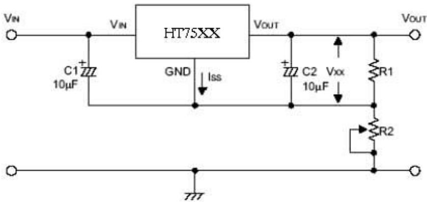
$$V_{OUT} = V_{XX} \left( 1 + \frac{R2}{R1} \right) + I_{SS} * R2$$
