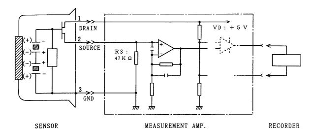
★ MEASUREMENT AMP.: NON-INVERTED TYPE, GAIN 72.5 dB AT 1 Hz 0.4~2.7 Hz/-3 dB
